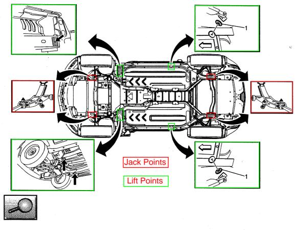
Caution: To avoid any vehicle damage, serious personal injury or death when major components are removed from the vehicle and the vehicle is supported by a hoist, support the vehicle with jack stands at the opposite end from which the components are being removed.
